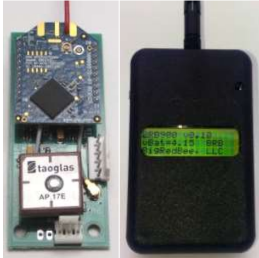
Figure 4 BRB900 GPS Receiver(L) and Transmitter(R)
