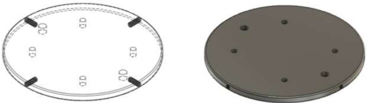
Figure 20 Aluminum Hub Bulkhead
