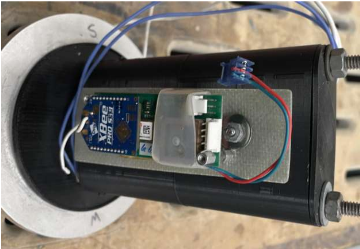
Figure 11 Hummingdoot V2 Phase 2 XBee GPS System
