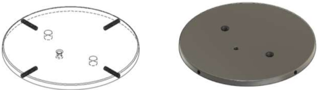
Figure 10 Aluminum Bulkhead model
